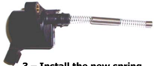
3 – Install the new spring conductor by pushing onto the coil's terminal. For COP boots with integral spring, install boot in same position as original and move onto step 5.
