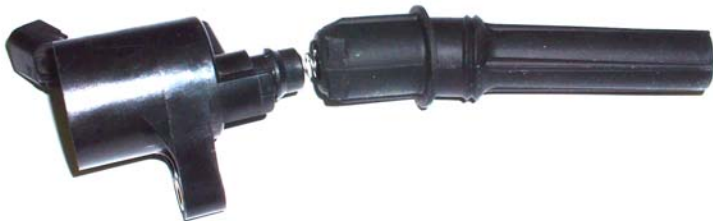
4 – Slide the new boot over the spring. Check for any alignment tabs on the coil, especially with angled boots, and slide firmly on.
